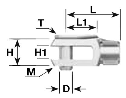
$\begin{array}{lll} D & = \varnothing 8, 1 \\ H & = 16 \\ H1 & = 8 \\ L & = 32 \\ L1 & = 16 \\ M & = Metal \\ T \ (Thickness) = 16 \end{array}$
